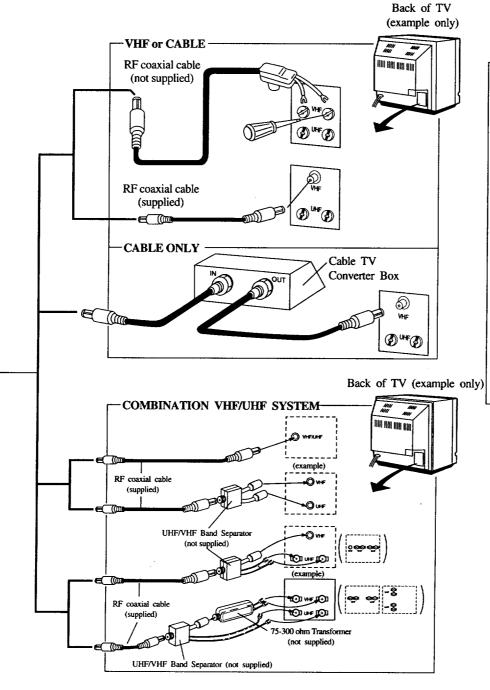
If you have a UHF-only antenna system: Even if you only plan to play tapes and view/record UHF channels, you still need to make one of the combination UHF/VHF connections shown. This is because when your VCR operates, it sends VHF signals to the TV across the RF coaxial cable. You may connect the cable TV converter box two different ways. See pages 38-39 before you choose how to connect the cable TV converter box.
